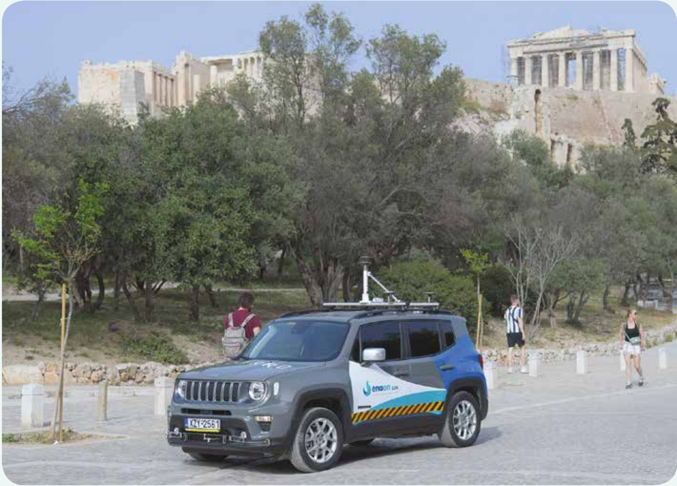
3. In 2023, Picarro technology was implemented in Greece to inspect approximately 9,000 km of pipelines, corresponding to 120% of the network.
